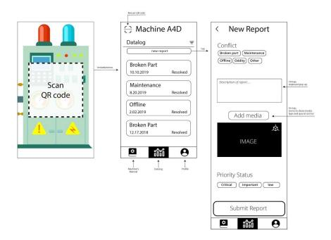
After scanning the QR code on the machine, the user will be brought to the main page showing all of the current and past issues for that specific machine.
